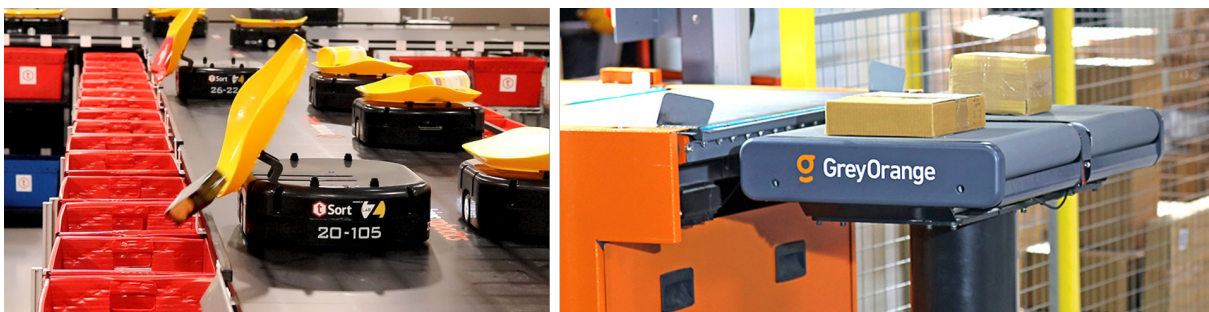
Figure 1 Robotized sorting systems t-Sort of Tompkins Robotics (left; source: Tompkins Robotics) and Ranger Mobile Sort of Grey Orange (right; source: Grey Orange).
