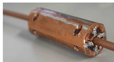
(b) Floating Cable Trap
