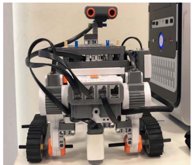
Figure 4: The Ultrasound sensor placed at the top of the model
