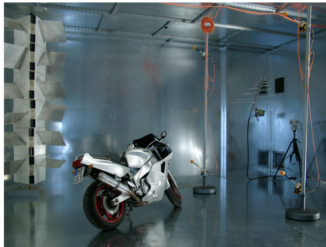
Figure 2.12: Photograph of the big reverberation chamber at the at OvGU [Wik20]
