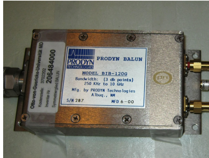
Figure 2.17: Photograph of a balancing unit for the measurements of e. g. a double wire in free space
