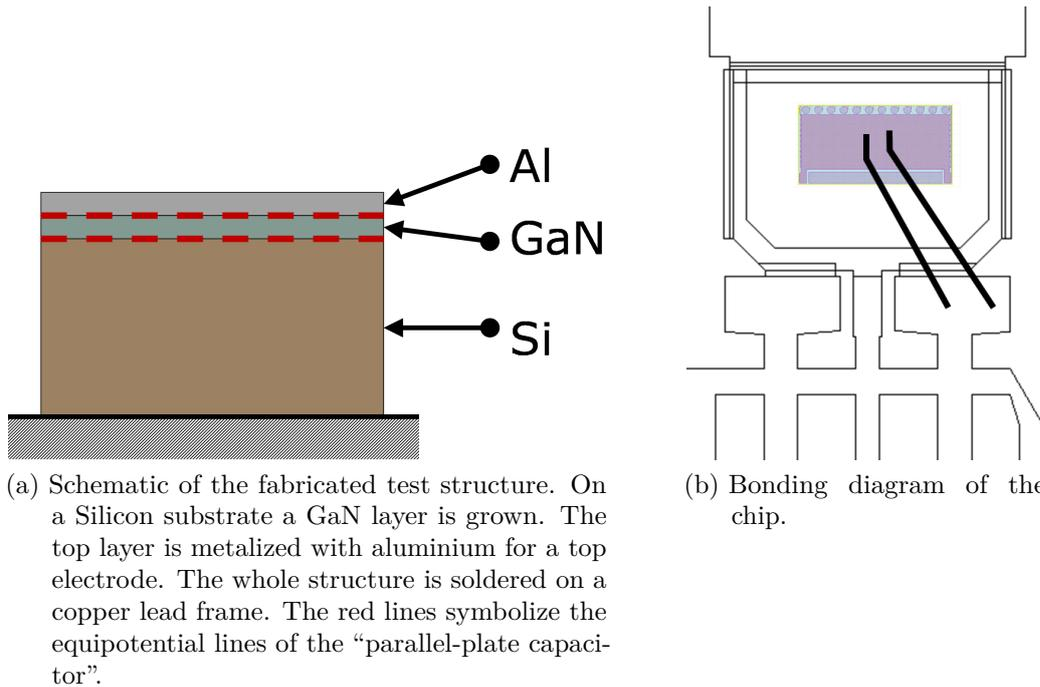
Figure 5.14: Schematics of the test chip.
