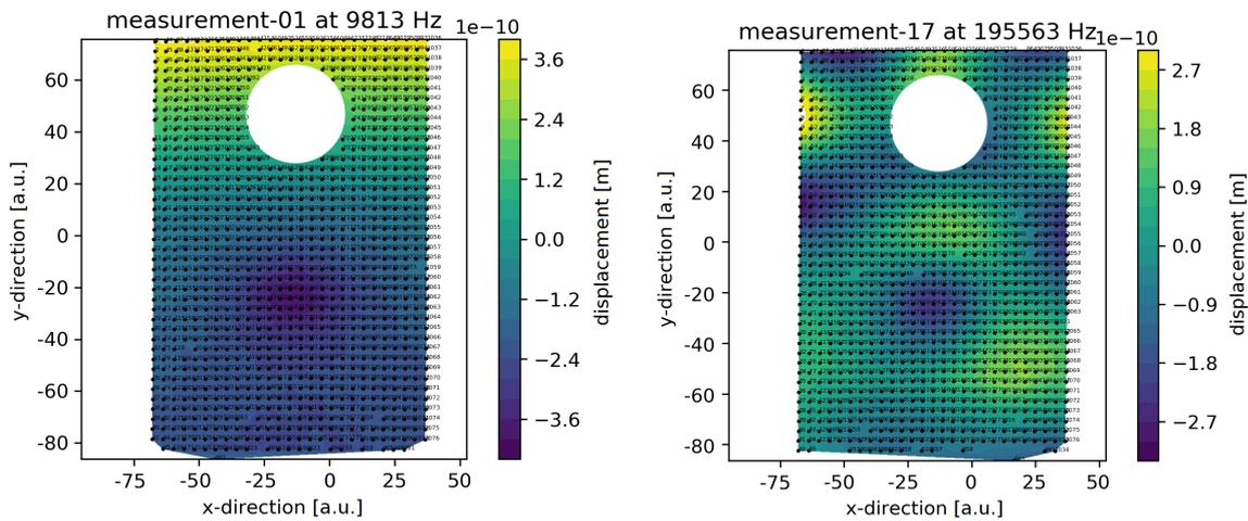
(a) Measurement of the eigenmode 1 at 9813 Hz. (b) Measurement of the eigenmode 17 at 195563 Hz.
