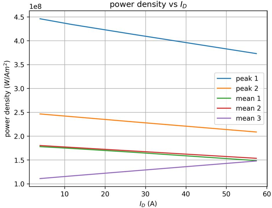
Figure 4.12: Linear regression of the power distribution in  $W/m^2$  for different current levels at  $V_{DS} = 400$  V.
