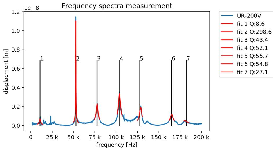
Figure 5.11: Analysis of the displacement spectral for the upper left reference point. All resonance peaks are fitted.
