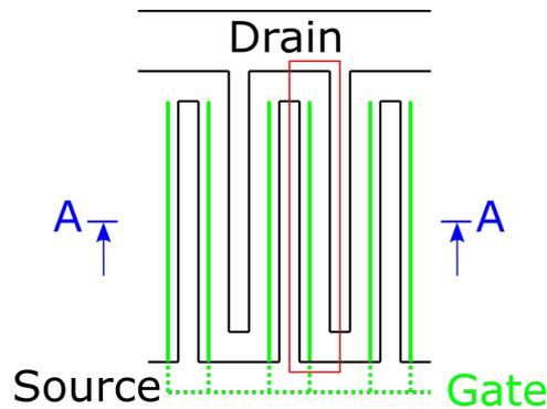
Figure 4.6: Schematic top view of a GaN HEMT, with highlighted drain, source and gate. The red rectangle marks one single cell. The neighbouring single cells show an antiparallel alignment. The gate bus, connecting all the gate fingers is below the big source pad on the bottom.
