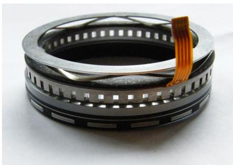
(a) Ultrasonic motor used in an auto focus objective in photography. [Ter08]
