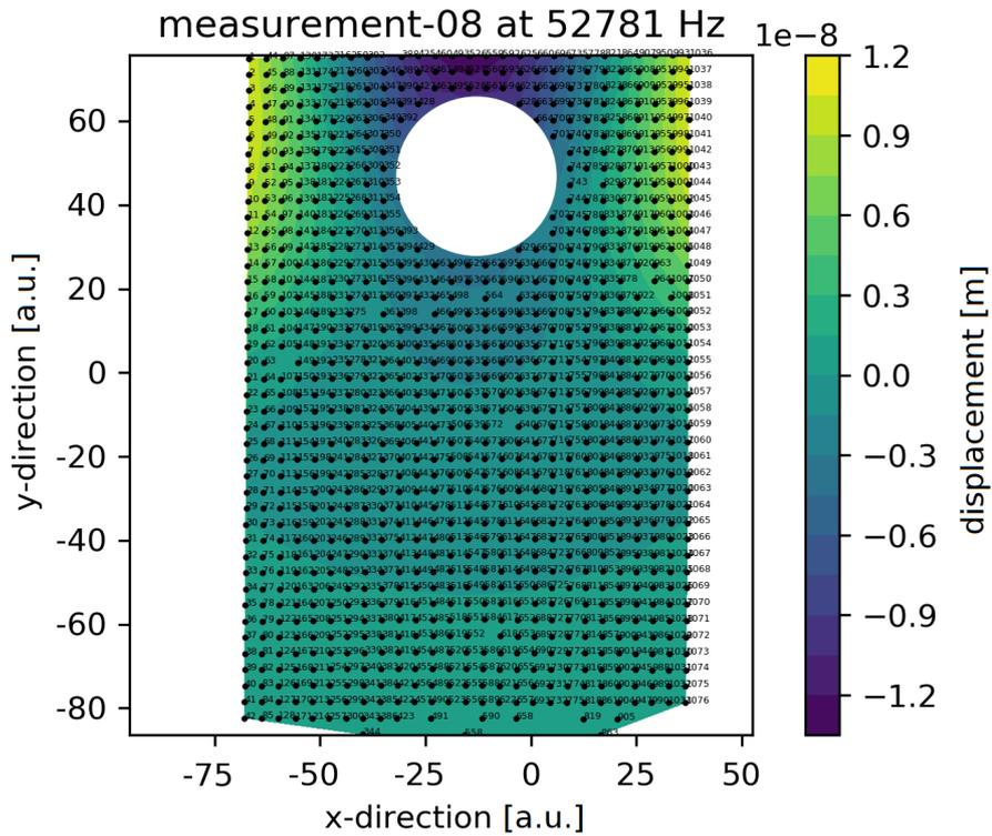
Figure 5.12: Scanning measurement of the resonance at 52781 Hz.
