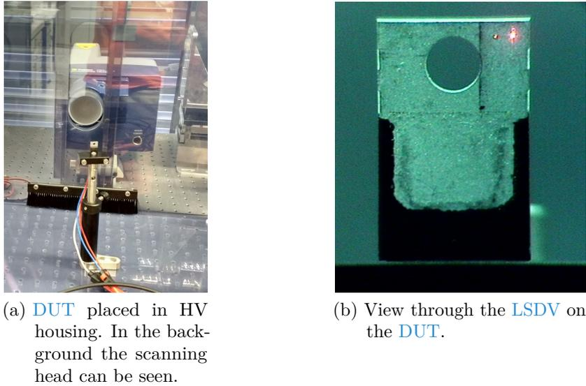
Figure 5.8: Measuring setup and view of the DUT through the LSDV.
