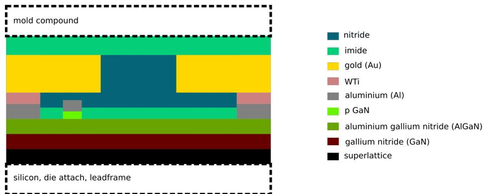
Figure 4.8: Schematic (not in scale) of a single GaN cell and the materials used.
