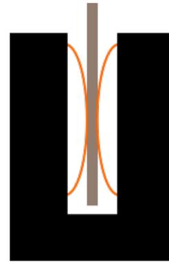
(b) Clamping principle of the socket.
