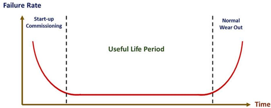
Figure 2.1: A bathtub curve describes the typical failure rate over time [Liv18].
