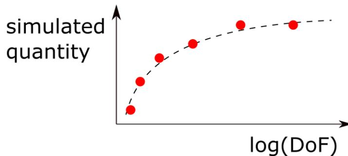
Figure 5.16: (Mesh) convergence of FEM models.
