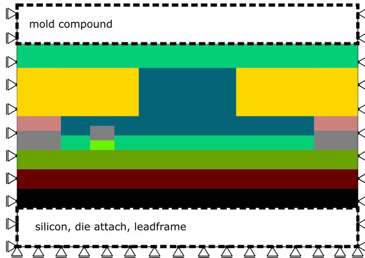
Figure 4.20: Mechanical boundary conditions of the single cell model.
