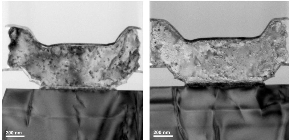
Figure 4.18: Bright field TEM images of reference (left) and with failed gate (right).
