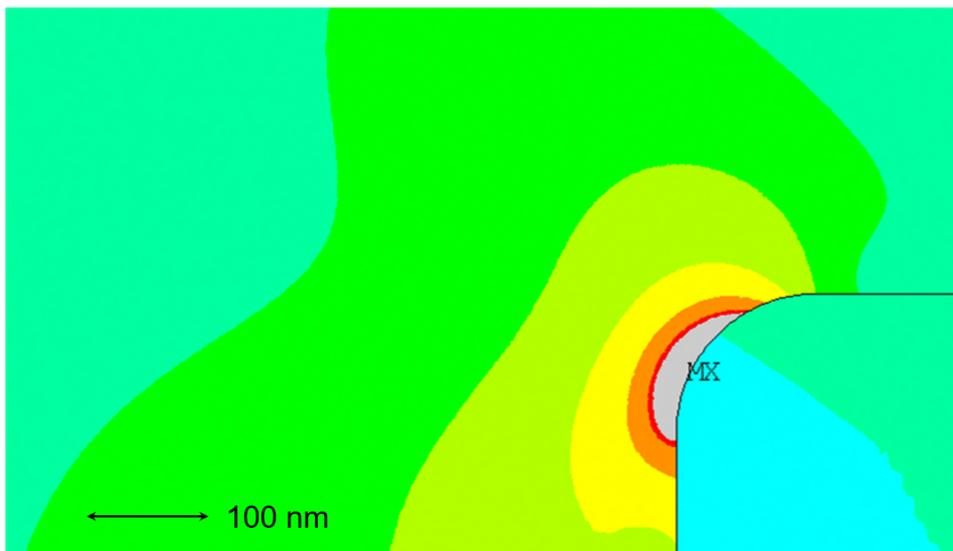
Figure 4.24: Magnification of stress on the gate edge facing the source side with a rounding of the edge.
