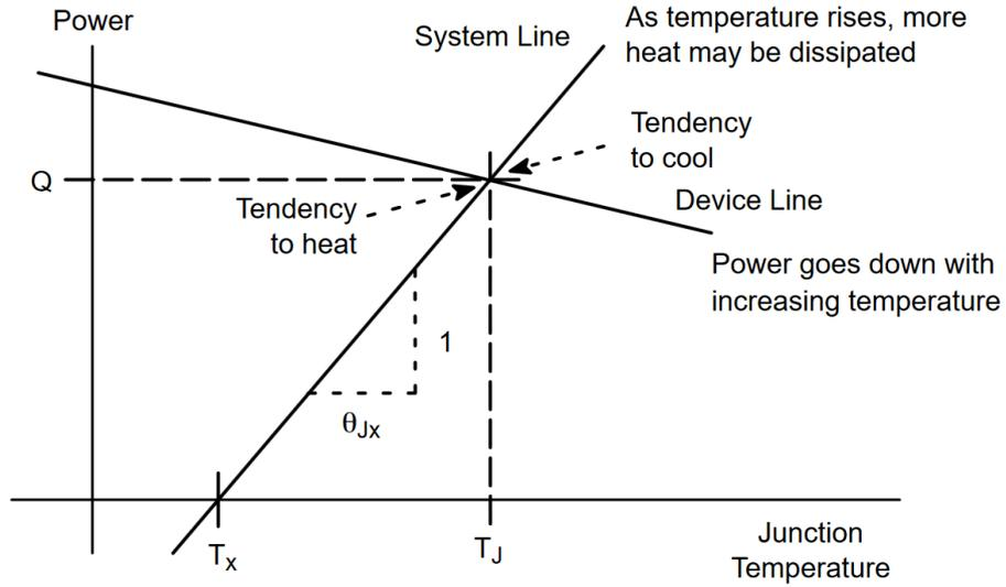
Figure 3.1: Example stability diagram of a thermal system. [Sto06]
