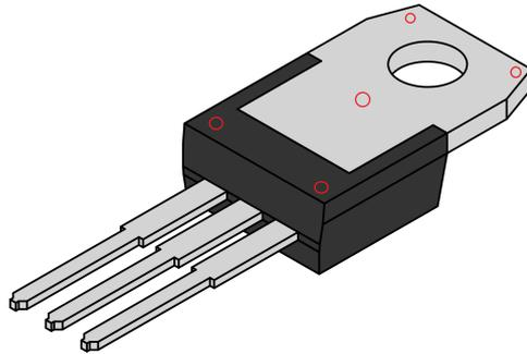
Figure 5.9: T0-220 backside view [Ind07].
