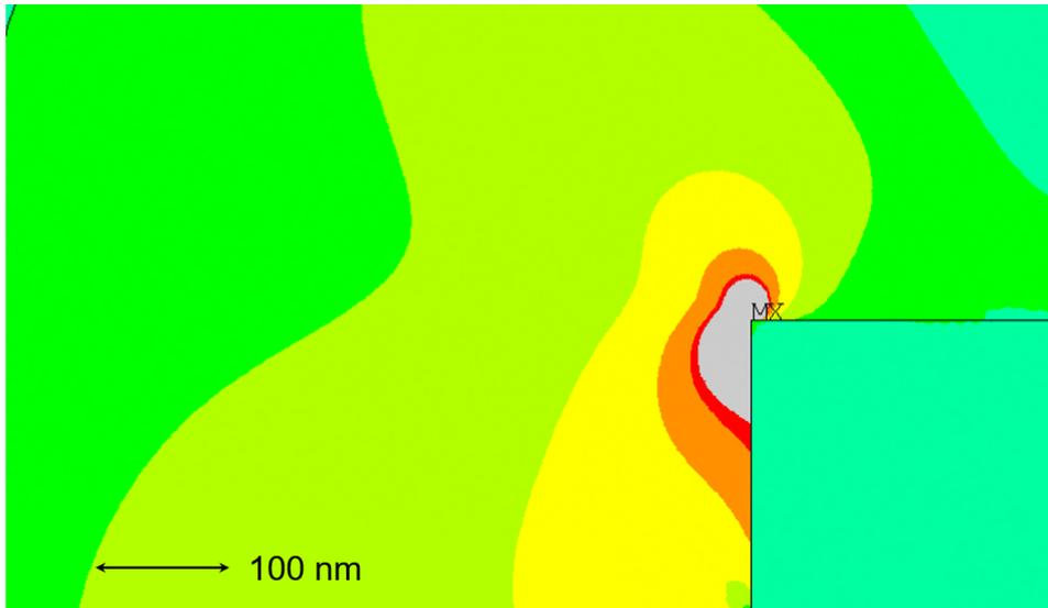
Figure 4.22: Magnification of stress on the gate edge facing the source side.
