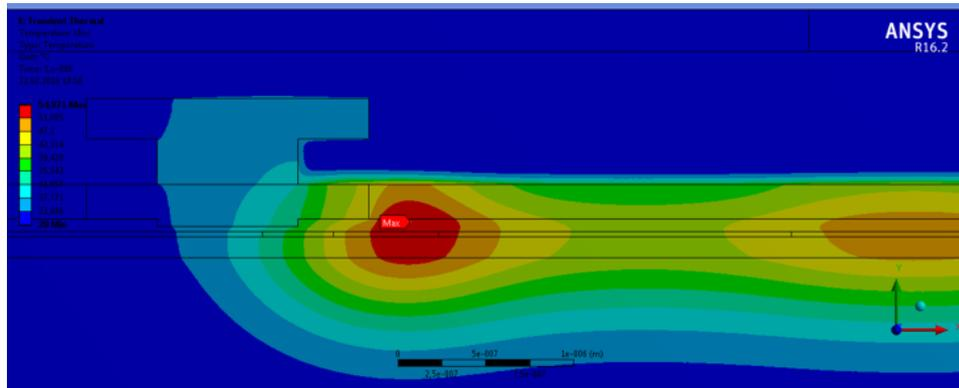
Figure 4.13: Exemplary temperature distribution at an arbitrary time within a pulse.
