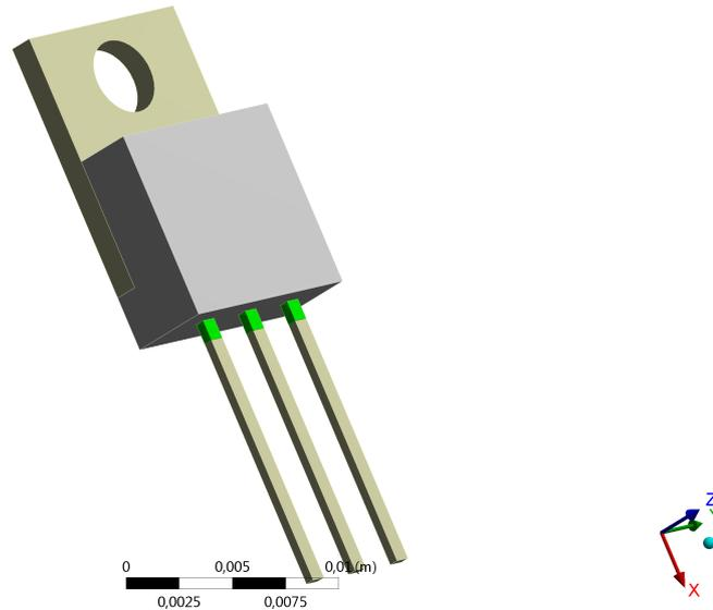
Figure 5.6: Model of a TO-220 package. The signal green part of the legs is free while the other part is fully clamped. The length of the green part has been varied to find the optimal free leg length.
