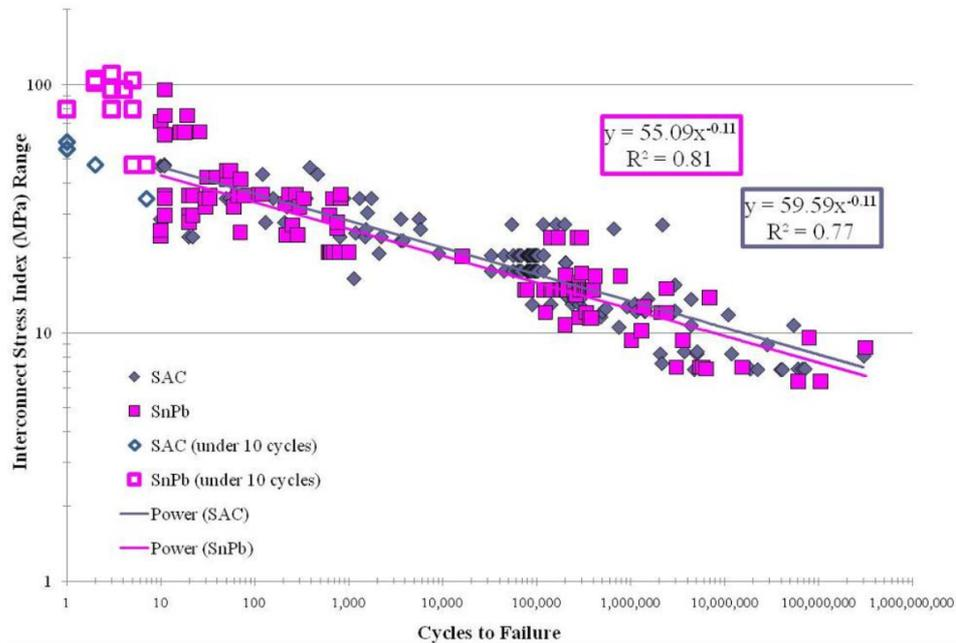
Figure 5.26: Exemplary SN curves of SnPb and SAC solder. [Paq10]
