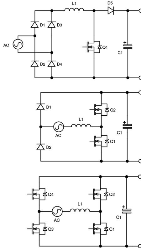
Figure 1.2: Schematics of an ordinary bridge rectifier with a boost converter evolving into a bridgeless totem pole PFC [Li20].
