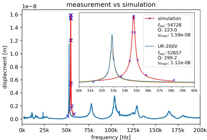
Figure 5.20: Result of the harmonic simulation. Each blue cross is the result of one single simulation. For easier visual inspection the blue crosses are fitted with the red line. The purple line is the measured deformation of the same point. (Orange depicts the fit of the measured result)
