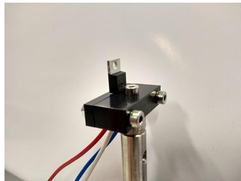
(b) Isometric view on the [DUT](#) in the new clamping vise.
