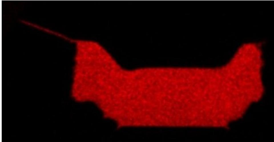
Figure 4.16: Elemental map at the point of protrusion. It can be clearly seen that the crack in the ILD is completely filled with aluminium from the gate finger causing an electric short between gate and source.
