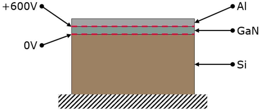
Figure 3.6: Stack to show the interaction of temperature and voltage.
