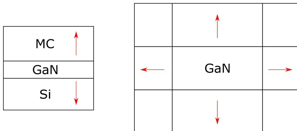
Figure 5.15: Meshing strategy for the test chip. The left figure shows the stack from a side view the right one a top view picture.
