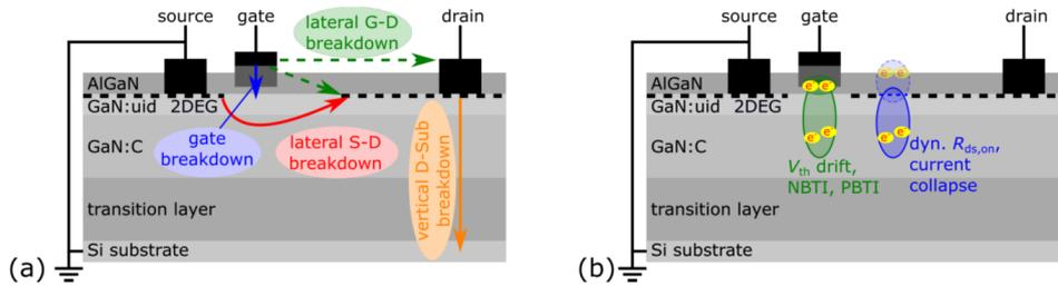
Figure 2.2: Possible break through paths of a GaN HEMT can be seen in figure (a), whereas (b) shows typical trapping sites and their effects [Kř20].
