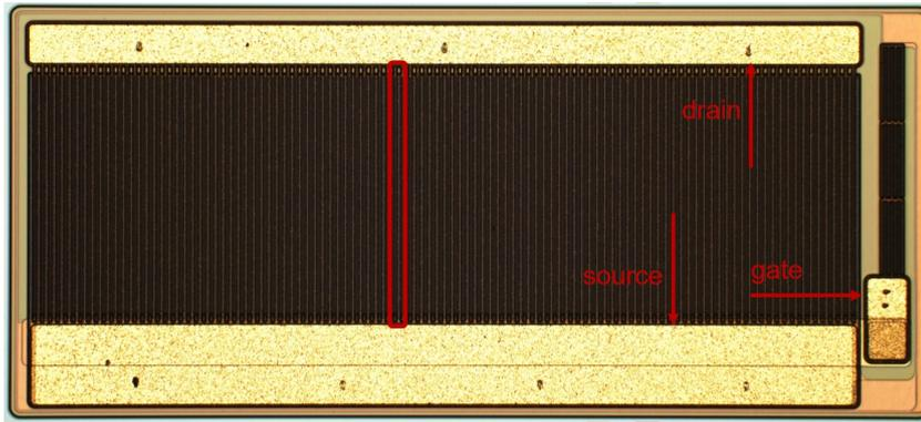
Figure 4.5: Topview of a GaN HEMT, with highlighted drain, source and gate pad. The red rectangle shows one single cell. The complete chip measures  $4.8 \times 2.2$  mm
