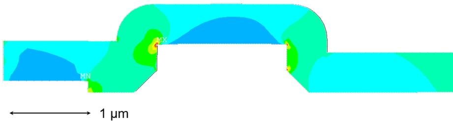
Figure 4.21: Overview of the stress in the ILD layer. It can be seen that the peak first principle stress areas are located on the gate edges. Compared to [Figure 4.19](#) or [Figure 4.18](#) that the geometry of the gate finger has been simplified without affecting the overall result.
