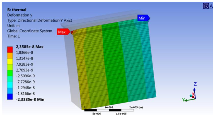
(b) y direction deformation of the full stack (relaxed at 293 K) is subjected to temperature increase  $\Delta T$  of 180 K
