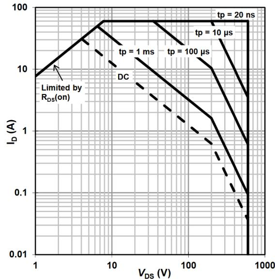
Figure 4.1: Principle SOA diagram of GaN HEMTs [18]. The SOA depends on the time of the pulse. For pulses with a duration of approximately 100  $\mu$ s, the applied  $V_{DS}$  and  $I_D$  are at least one order of magnitude away from their rated limits.
