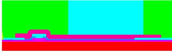
Figure 4.7: Model of a single GaN cell (section view AA from Figure 4.6). The source is located on the left, whereas the drain is the right. The colors mark different materials.
