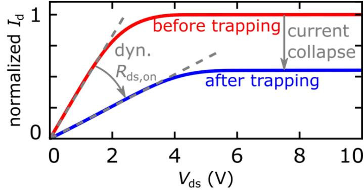
Figure 2.3: Effects of current collapse and dynamic  $R_{ds,on}$  on the drain current with respect to the gate source voltage [K̃T̃20].
