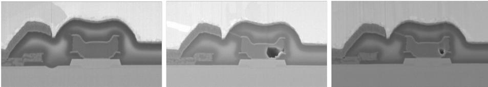
Figure 4.15: Series of three **SEM** pictures after **FIB** cuts along the gate finger axis (normal to the picture plane) showing the beginning middle and end of the point of failure
