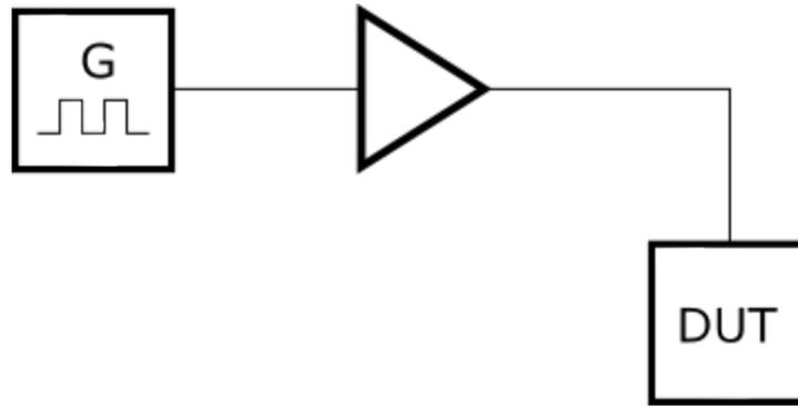
Figure 5.2: Principal circuit diagram of the excited DUT.
