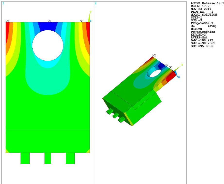
Figure 5.17: Exemplary result of the modal analysis, where the swinging form of the 10<sup>th</sup> eigenmode at a frequency of 54 969.9 Hz is shown. (For the color code note that red marks the maximum positive deflection, while blue marks the minimum deflection)
