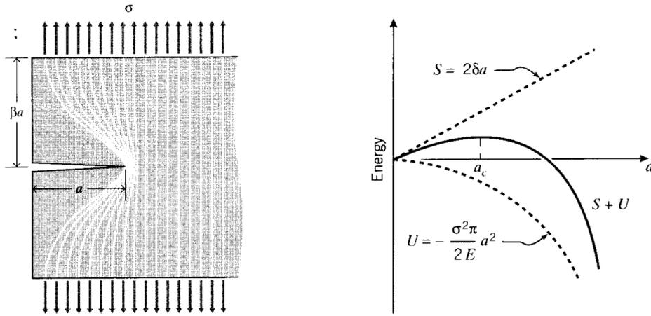
(a) Plate with pre-crack. The roughly triangular stress free area can be seen to both sides of the crack
