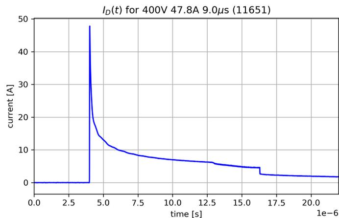
Figure 4.4: Exemplary  $I_D(t)$  of a sample short circuit pulse for a constant  $V_{DS}$  of 400 V.  $V_{GS}$  was held for 1 ms. As can be seen the short between gate and source forces the device in an off state much earlier.
