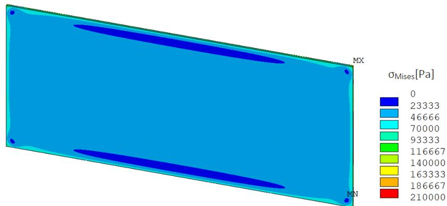
Figure 5.27: Von Mises stress of the die attach layer.
