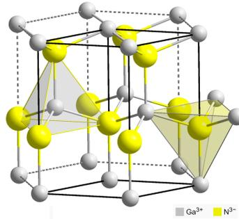
Figure 1.1: GaN Wurtzite structure [08]
