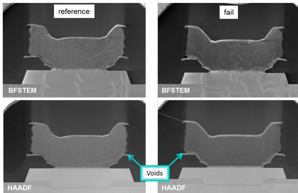
Figure 4.19: STEM and HAADF of gate area. The left picture shows a reference chip, whereas the right one shows a failed region.
