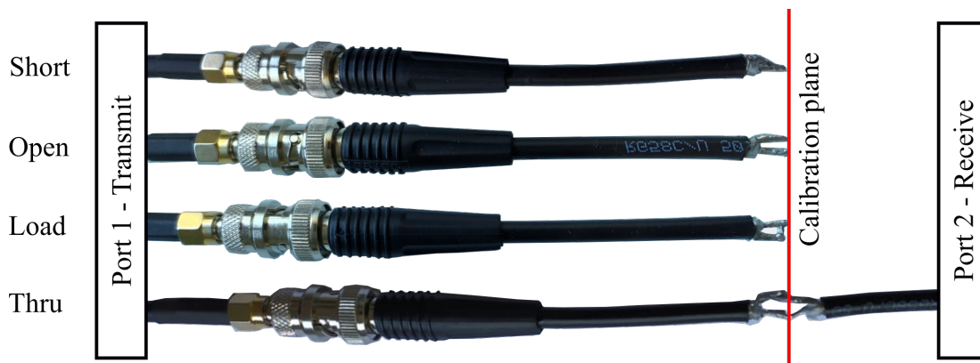
Figure 2.7: Before the VNA can be used, it must be calibrated. During calibration, the power cable is not connected to the adapters. The figure shows the calibration scheme using the adapters.
