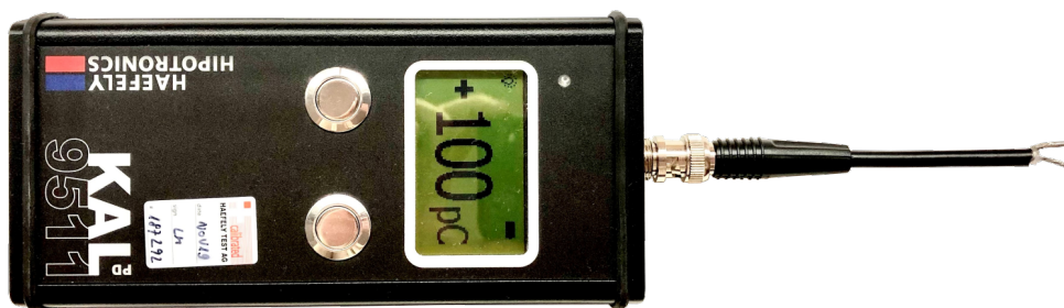
Figure 2.10: PD calibrator with adapter to connect to the power cable. An optional resistor R_{t1} can be soldered between the separated conductors to adjust the termination resistance Z_1 of the power cable if necessary. The oscilloscope is connected in a similar way.
