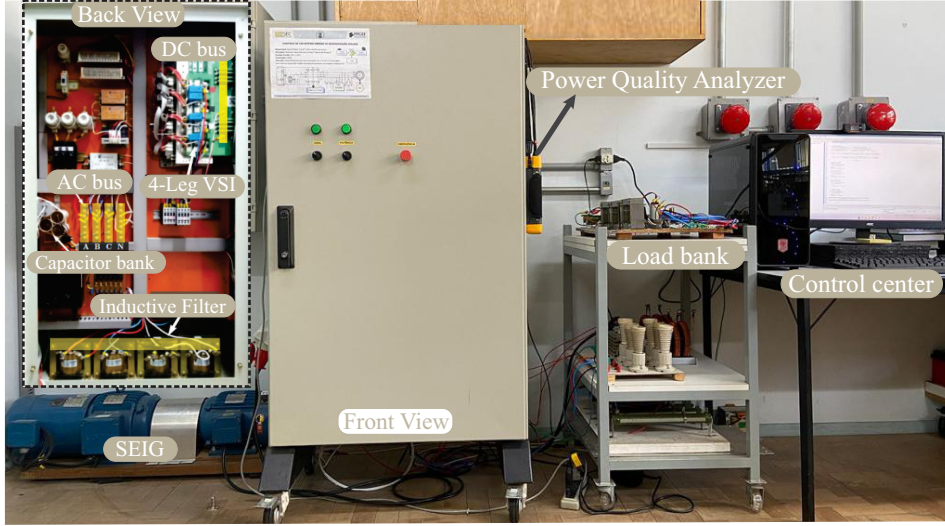
Figure G.1: Experimental setup
