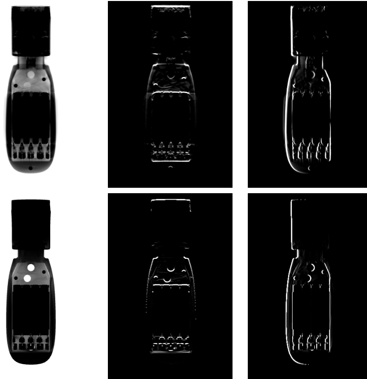
Figure 6.1: Exemplary comparison between a ray-casting DRR (upper row) and a DRR based on mesh-rendering (lower row) from the same point of view. The real DRR is shown on the left, horizontal edge images are shown in the middle, vertical edge images on the right.
