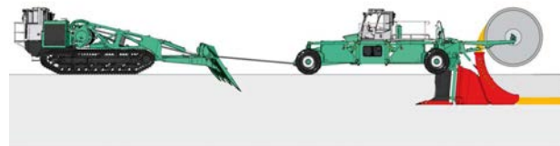
Fig. 2: Elements of Föckersperger cable laying system, from [17]
