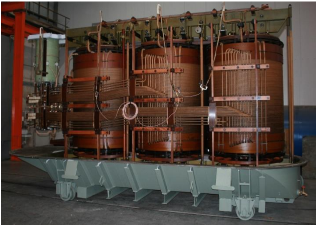
Fig. 7. Dried 25 MVA transformer
