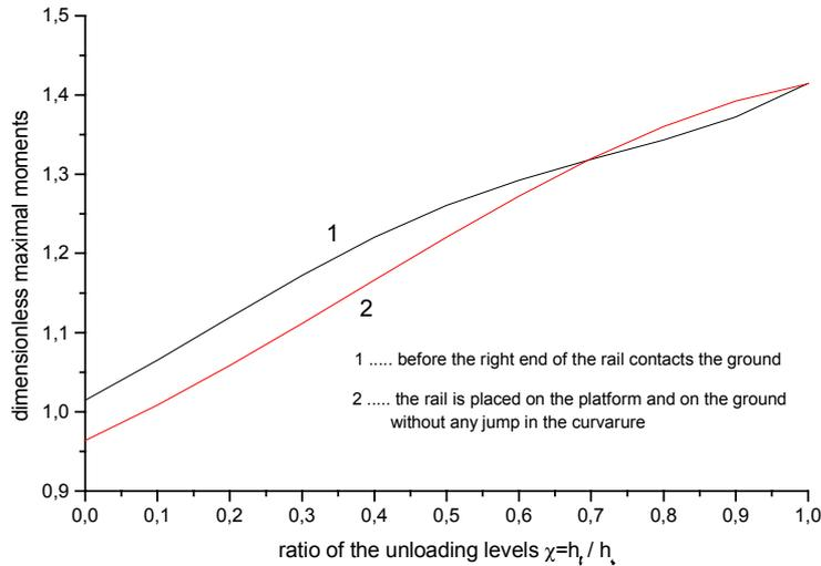
Figure 2: Dimensionless Moments  $\tilde{M}_0^u, \tilde{M}_0^m$  as a Function of the Ratio of the Unloading Levels  $\chi = h_\ell / h_r$  .
