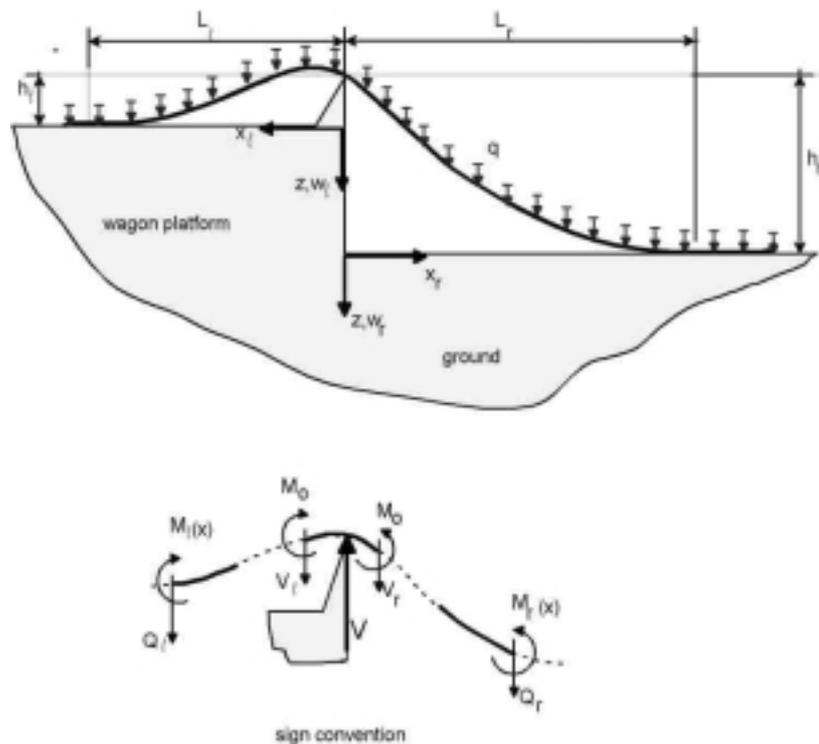
Figure 1: Schematic Representation of the "Mounting" Condition and the Definitions.
