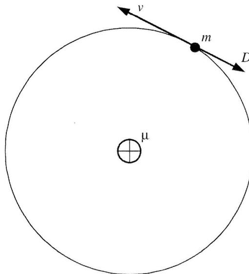
Figure 2. Satellite Velocity and Drag
