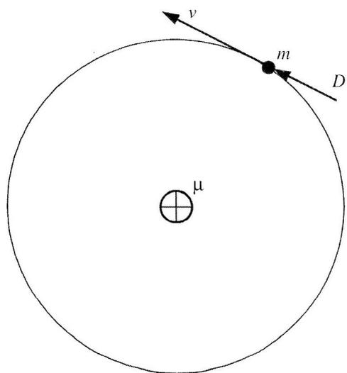
Figure 4. Satellite Velocity and Forward Thrust
