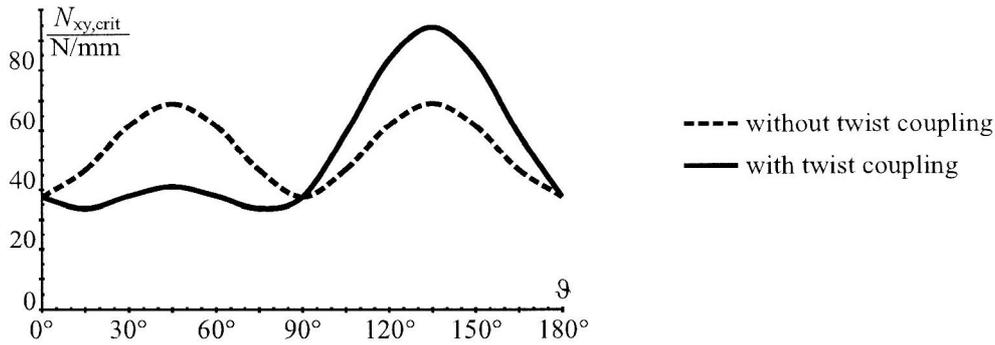
Figure 7: Critical Buckling Load  $N_{xy,crit}$  (in N/mm) for Simply Supported  $[\vartheta / -\vartheta / \vartheta / -\vartheta / \vartheta]$  Laminate Plate under Pure Shear Loading
