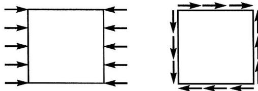
Figure 3: Considered Buckling Load Cases for Rectangular Laminate Plate
