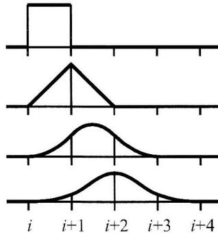
Figure 2: Normalized B-Splines of the Orders 1 to 4
