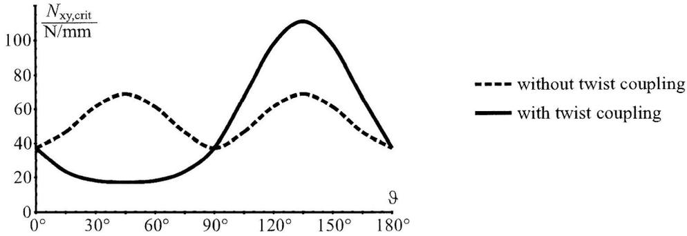
Figure 5: Critical Buckling Load  $N_{xy,crit}$  (in N/mm) for Simply Supported Single Layer Plate under Pure Shear Loading
