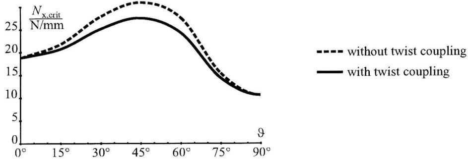
Figure 6: Critical Buckling Load  $N_{x,crit}$  (in N/mm) for Simply Supported  $[\vartheta / -\vartheta / \vartheta / -\vartheta / \vartheta]$  Laminate Plate under Uniaxial Compressive Loading
