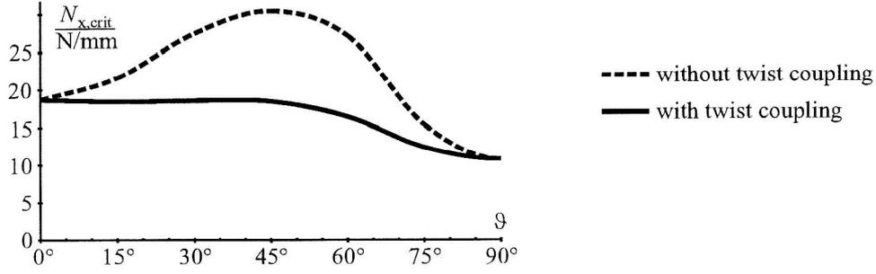
Figure 4: Critical Buckling Load  $N_{x,crit}$  (in N/mm) for Simply Supported Single Layer Plate under Uniaxial Compressive Loading
