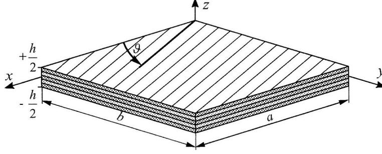
Figure 1: Considered Laminate Plate
