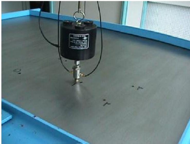
Figure 6. Steel Plate, Support, and Excitation
