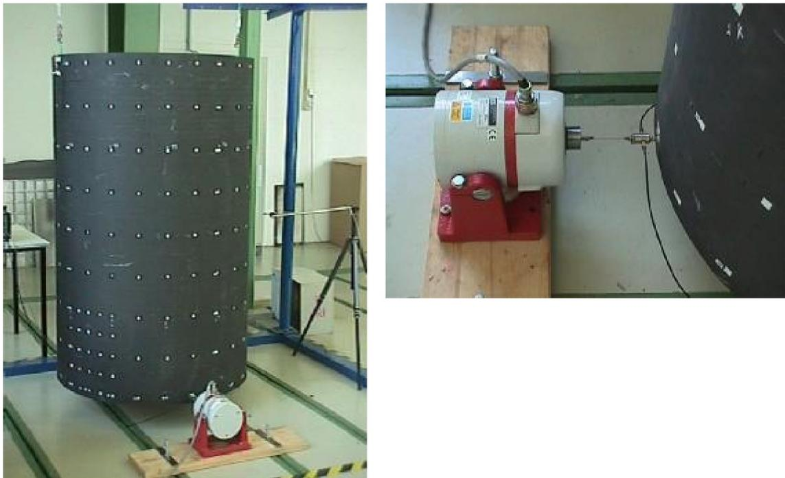
Figure 8. CFRP-Cylinder with Coupled Exciter
