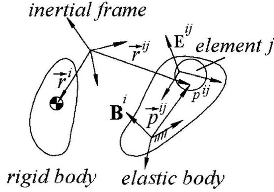
Figure 1. Multi Body System Consisting of Elastic and Rigid Bodies
