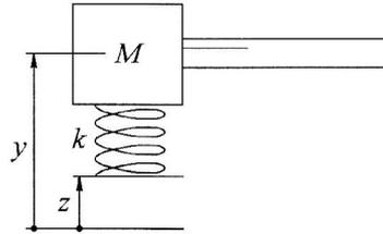
Figure 2. Lumped Mass, Cantilever Beam and Spring
