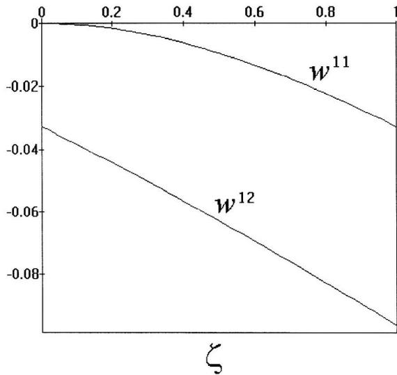
Figure 4. First Mode Shape of First and Second Element ( $\eta_1 = 1$ )
