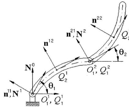
Figure 8. A two-Degree-of-Freedom Flexible Robot
