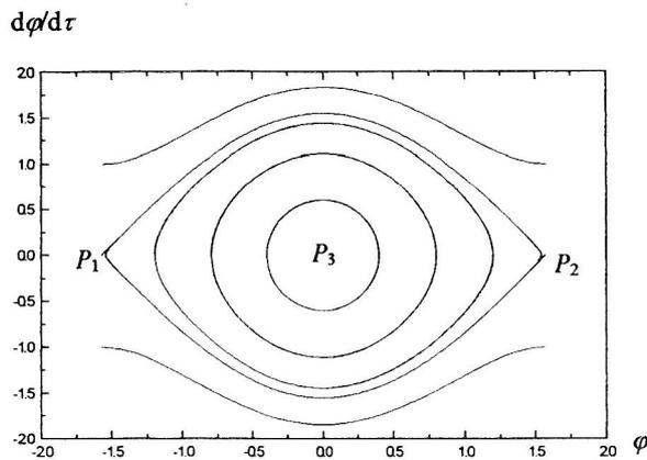
Figure 3. Phase Trajectories of Unperturbed System
