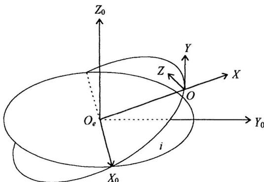
Figure 1. Inertial Coordinate System and Orbit Coordinate System
