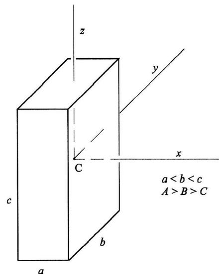
Figure 2. Model of an Asymmetric Gyro
