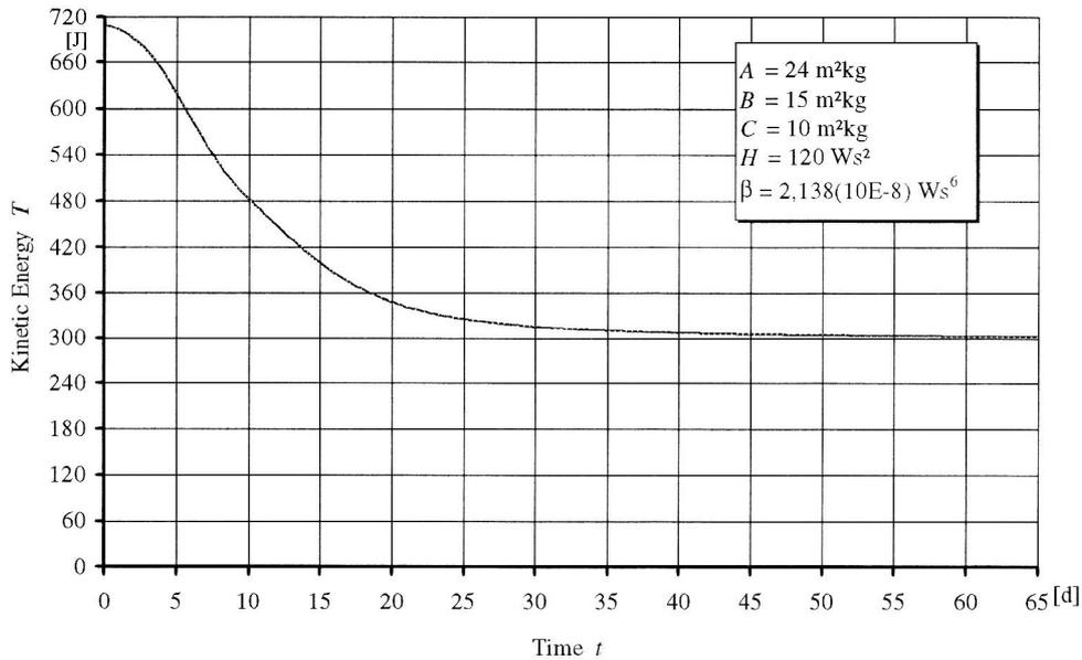
Figure 5. Decay of Kinetic Energy to its Minimum Value of  $T = H^2 / 2A$
