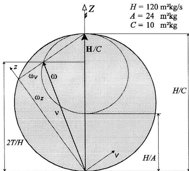
Figure 1. Attitude Diagram for an Axisymmetric Gyro
