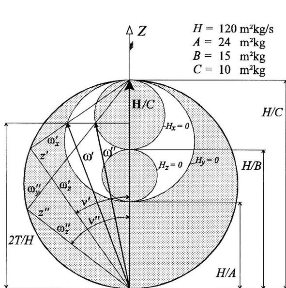
Figure 3. Attitude Diagram for an Asymmetric Gyro, Epicyclic Condition,  $H^2/2B < T < H^2/2C$
