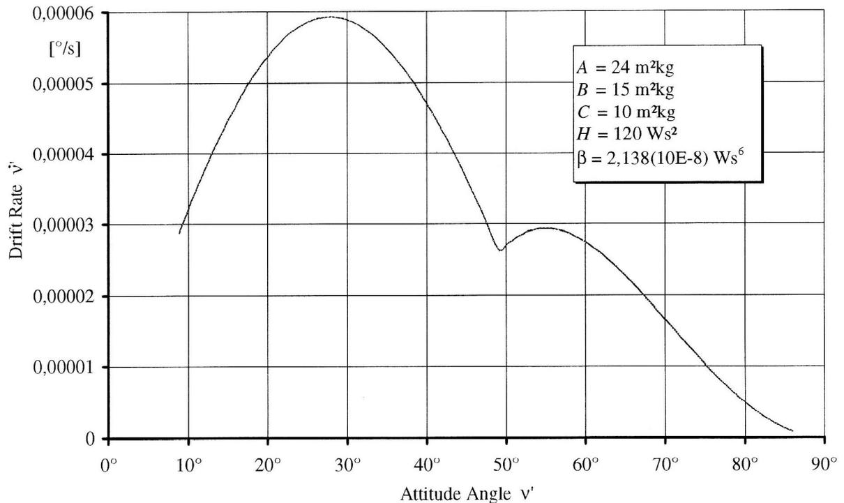
Figure 7. Attitude Drift Rate  $\dot{\nu}'$  as Function of Attitude Angle
