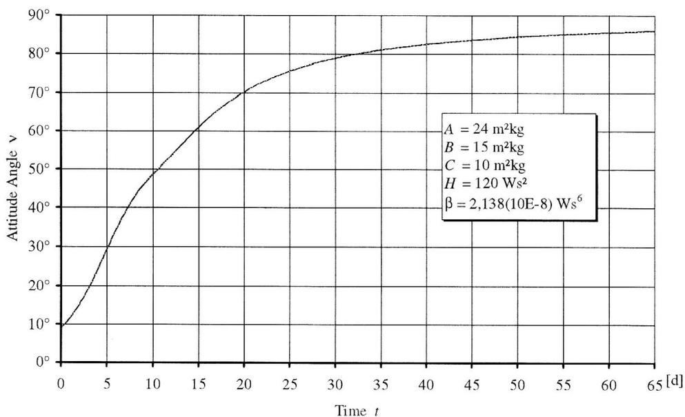
Figure 6. Increase of Attitude Angle towards its Final Value of  $\nu' = 90^\circ$
