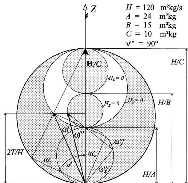
Figure 4. Attitude Diagram for an Asymmetric Gyro, Pericyclic Condition,  $H^2/2A < T < H^2/2B$
