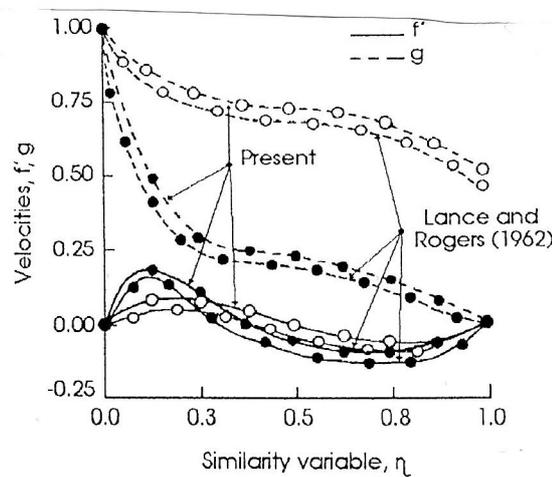
Figure 1. Radial and Tangential Velocity Profiles for •  $S = 0$ ,  $Re = 81$  and ◦  $S = 0.5$ ,  $Re = 25$
