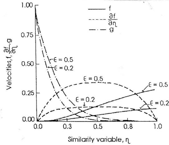
Figure 2. Axial, Radial and Tangential Velocity Profiles at  $t^* = 1$  for  $\phi(t^*)$ ,  $M = 4$  and  $Re = 25$
