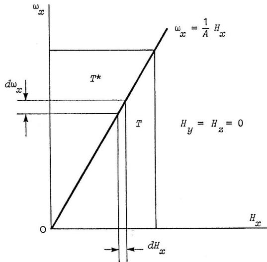
Figure 1. Kinetic Energy  $T$  and Kinetic Coenergy  $T^*$
