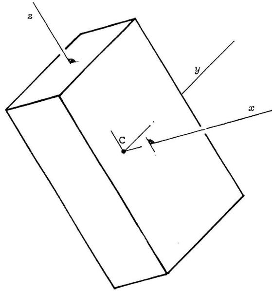
Figure 2. Rectangular Body with Uniformly Distributed Mass,  $A > B > C$ , Mass Centre  $C$ , and Body-fixed  $Cxyz$  Coordinates
