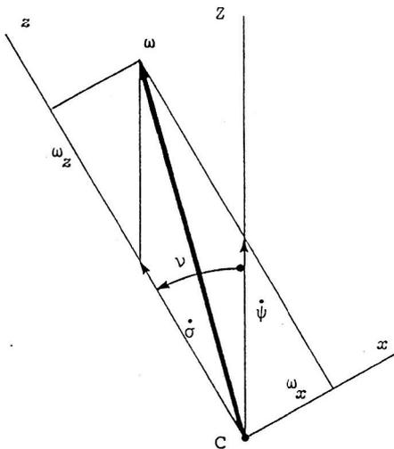
Figure 11. Angular Velocity at the moment where  $\omega_y = 0$
