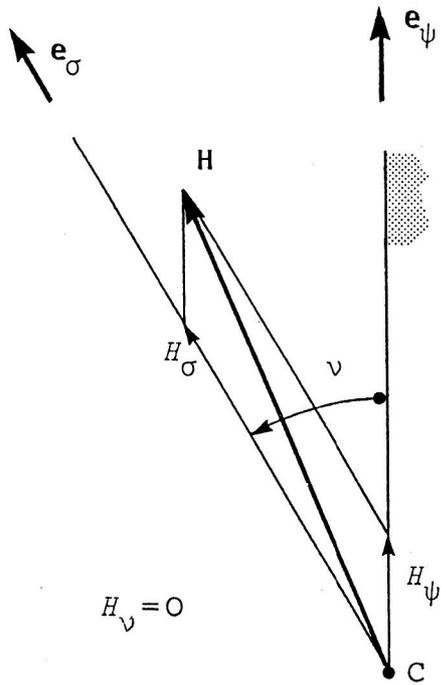
Figure 7. Contravariant Components of the Angular Momentum
