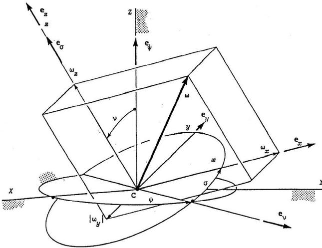
Figure 3. Position of Gyro-fixed  $Cxyz$  Coordinates in Euler Angles, and Angular Velocity  $\omega$
