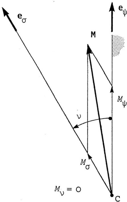
Figure 9. Contravariant Components of the Torque
