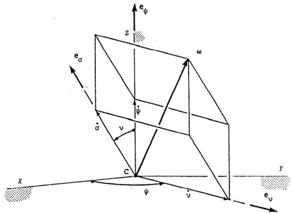
Figure 4. Eulerian Contravariant Components of the Angular Velocity
