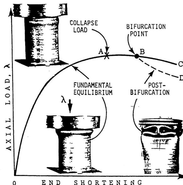
Figure 2. Load-end shortening curve with limit point A, bifurcation point B, and post-buckling equilibrium path BD (from Bushnell, 1985)
