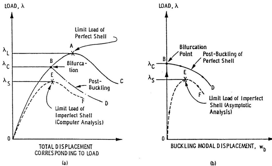
Figure 3. Load deflection curves showing limit and bifurcation points (from Bushnell, 1985)
