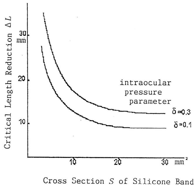
Figure 2. The critical length reduction of a silicone band vs its cross sectional area
