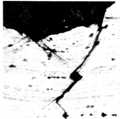
Fig. 5 Localisation of flow in underaged aluminium alloy (courtesy Dr. J. J. Lewandowski)
