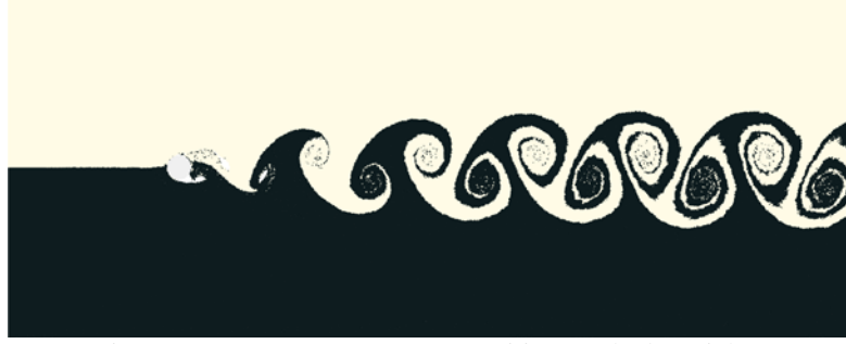
Figure 4. Karman vortex street (position marked particles)
