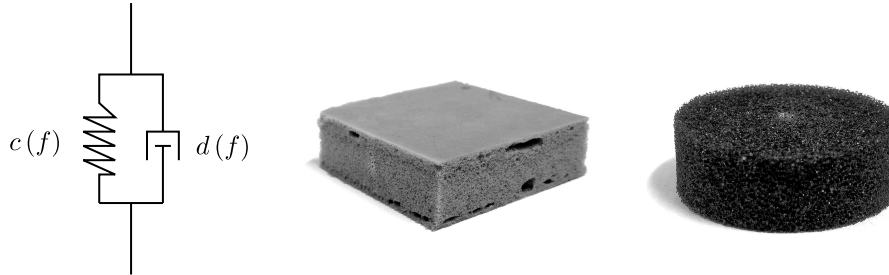
Fig. 1: Viscoelastic representation of the material behaviour (left) and foam samples B□50.x (center) and D○30.x (right).
