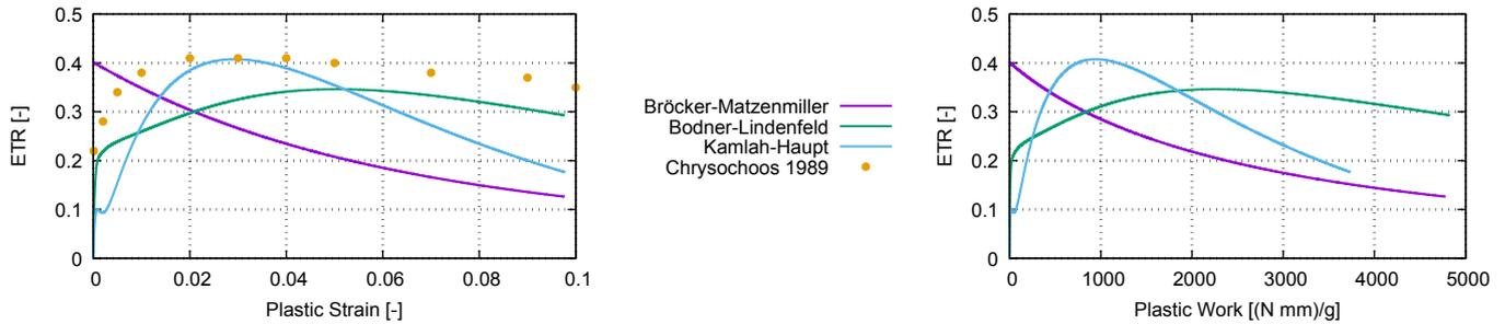
Fig. 4: Energy transformation ratio over plastic strain (*left*) resp. plastic work (*right*) for a uni-axial tension (XCrNi18.9 stainless steel)
