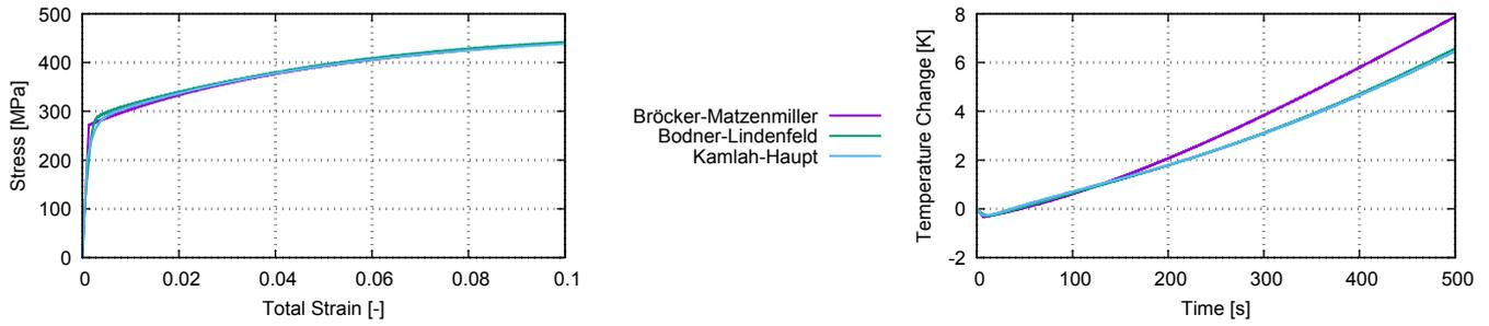
Fig. 3: Stress-strain curves (*left*) and temperature evolution (*right*) for a uni-axial tension (XCrNi18.9 stainless steel)
