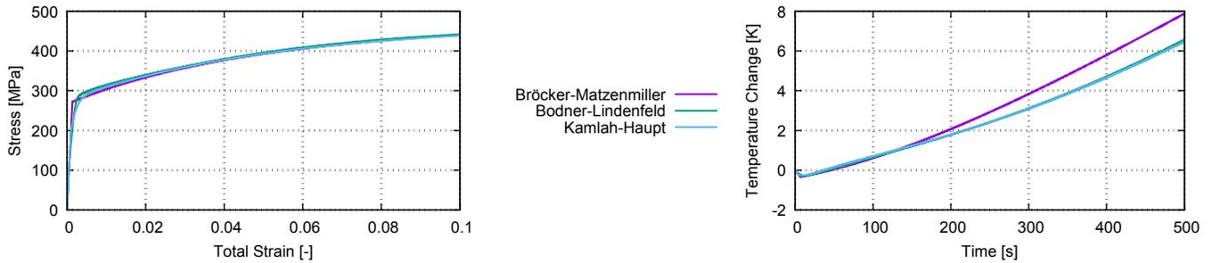
Fig. 3: Stress-strain curves (*left*) and temperature evolution (*right*) for a uni-axial tension (XCrNi18.9 stainless steel)
