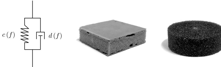
Fig. 1: Viscoelastic representation of the material behaviour (left) and foam samples B□50.x (center) and D○30.x (right).
