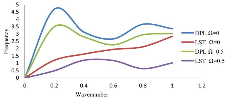
Fig. 2: Distribution of non-dimensional frequency against the wave number with and without of rotation.
