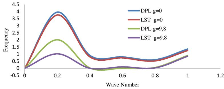
Fig. 1: Distribution of non dimensional frequency against the wave number with and without of gravity.
