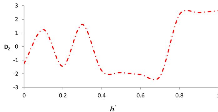
Fig. 11: Variation of electric displacement versus thickness of the coating material  $h'$  for  $[g=9.8, \Omega=0.5]$ .
