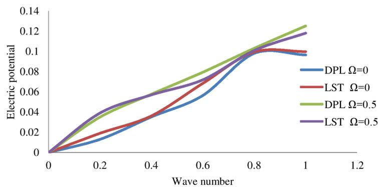
Fig. 6: Distribution of electric potential against the wave number in the absence and presence of rotation.
