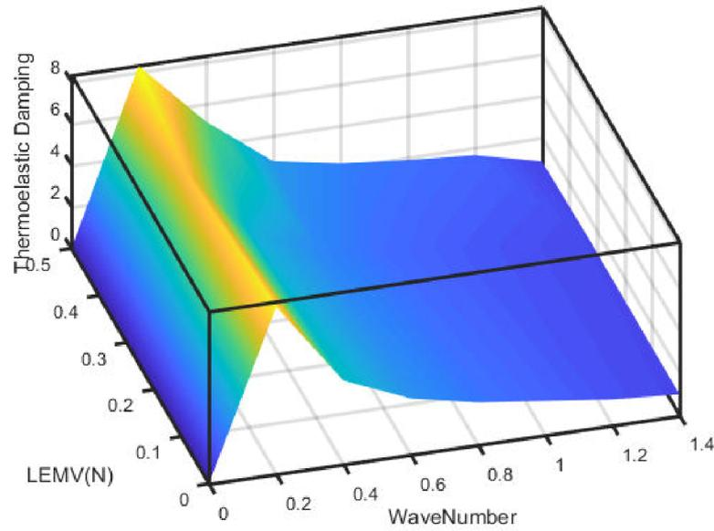
Fig. 8: Distribution of thermal damping against the wave number in the various values of CFRP (N) [g=9.8,Ω=0.5].
