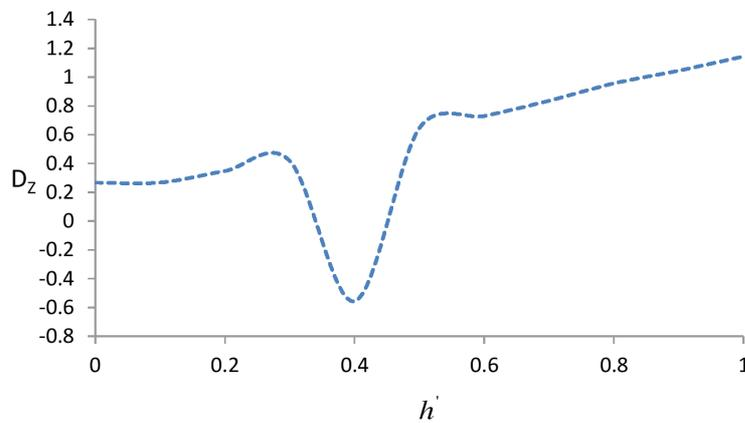
Fig. 9: Variation of electric displacement versus thickness of the coating material  $h'$  for [g=9.8,Ω=0]
