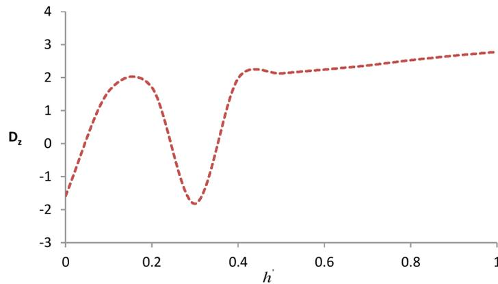
Fig. 10: Variation of electric displacement versus thickness of the coating material for  $[g=9.8, \Omega=0.2]$ .
