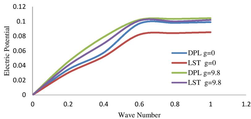
Fig. 5: Distribution of electric potential against the wave number with and without of gravity.
