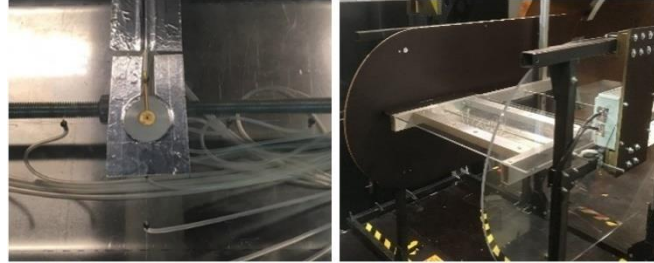
Fig. 5: Isolated static pressure probe on the test device
