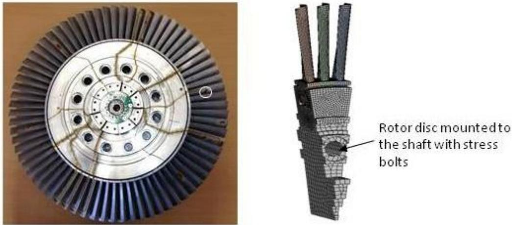
Figure 2. Rotor strain gauge application and FE model
