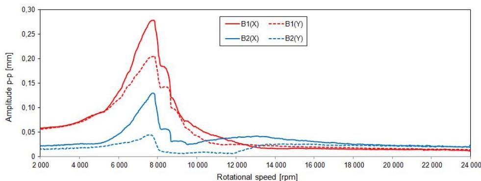
Figure 8. Peak-to-peak vibration amplitude of the shaft vs. rotational speed at 100°C (B1 – bearing no. 1, B2 – bearing no. 2, X – horizontal direction, Y – vertical direction)
