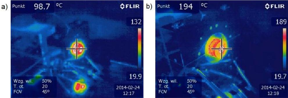
Figure 4. Foil bearing temperature measured using a thermal imaging camera: a – temperature on the external part of the journal, b – temperature in the journal opening
