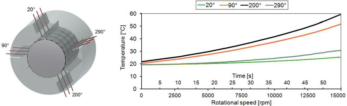
Figure 3. Thermocouples' location (left) and measured temperature of the central part of the foil bearing during acceleration of the rotor (right)
