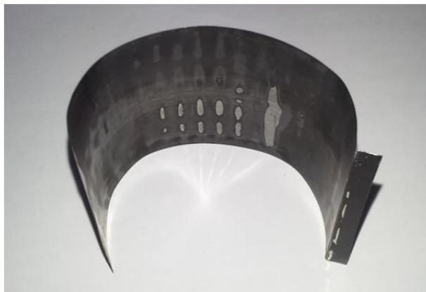
Figure 5. Damage of the sliding surface in the top foil
