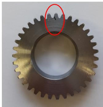
Figure 2: Artificially cracked planet tooth
