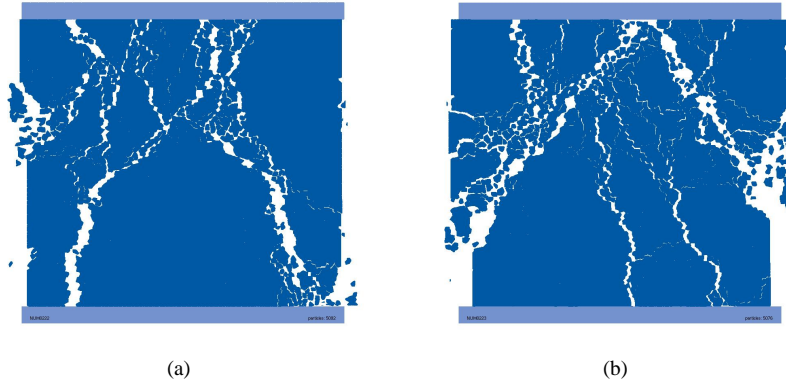
Figure 3: Crack patterns and failure of the concrete specimen in the DEM simulation
