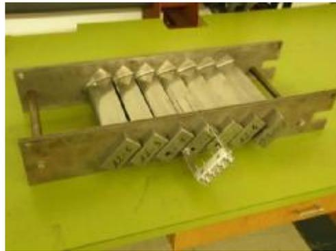
Figure 3: Turbine blade cascade
