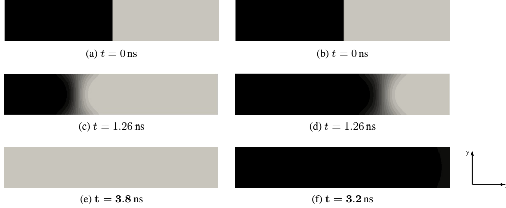
Figure 4: interface motion for a two-phase beam, black: austenite, white: martensite (a),(c),(e): T = 100 K, (b),(d),(f): T = 1300 K
