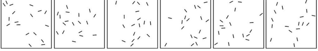
Figure 3. Random microstructure realizations with volume fraction = 0.1%, Fiber Length = 3.27 mm
