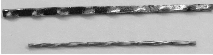
Figure 8. Surface deformities can be introduced into fibers during manufacturing to improve bond performance between the fiber and matrix. Common methods include crimping (top) and twisting (bottom)
