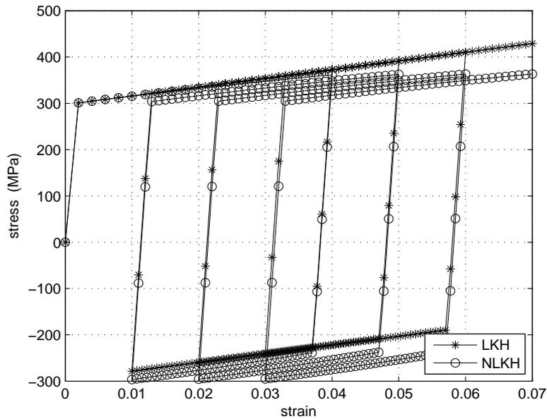
Figure 6: Comparative analysis between linear kinematic hardening (LKH) and nonlinear kinematic hardening (NLKH) in plasticity for carbon steel Ck 15. Loading conditions with increasing levels of loading and with loading program reported in Fig.3.
