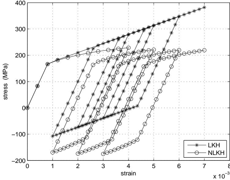
Figure 4: Comparative analysis between linear kinematic hardening (LKH) and nonlinear kinematic hardening (NLKH) in plasticity for chromium-nickel stainless steel X5CrNi 18.9. Loading conditions with increasing levels of loading and with loading program reported in Fig.3.
