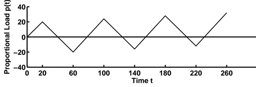
Figure 1: Loading program in tension-compression with increasing mean stress.
