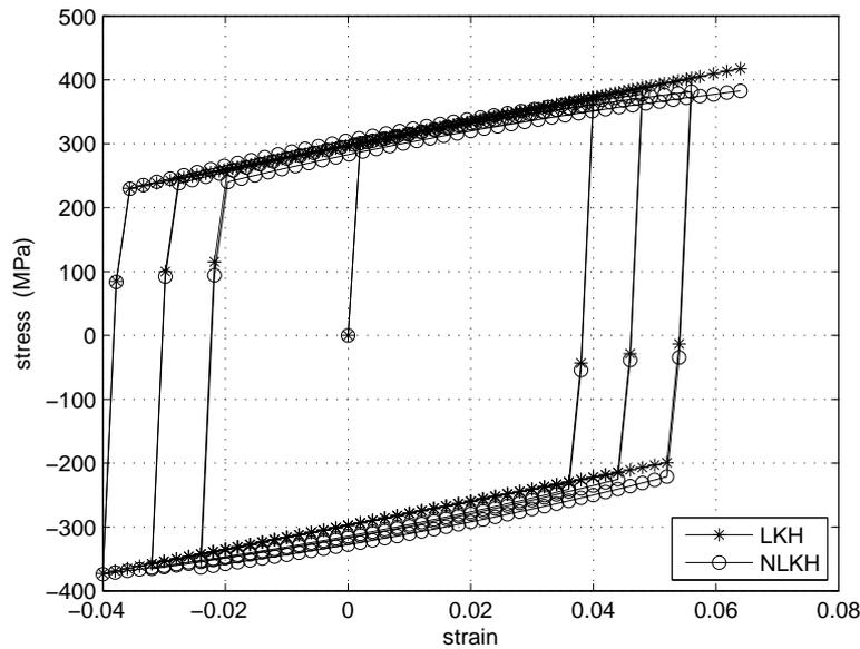
Figure 5: Comparative analysis between linear kinematic hardening (LKH) and nonlinear kinematic hardening (NLKH) in plasticity for carbon steel Ck 15. Loading conditions in tension-compression with loading program reported in Fig.1.
