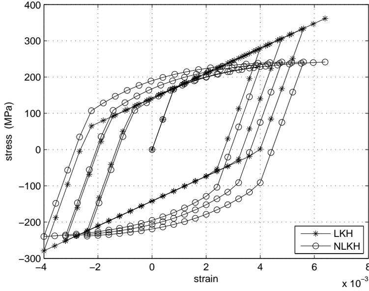
Figure 2: Comparative analysis between linear kinematic hardening (LKH) and nonlinear kinematic hardening (NLKH) in plasticity for chromium-nickel stainless steel X5CrNi 18-9. Loading conditions in tension-compression with loading program reported in Fig.1.
