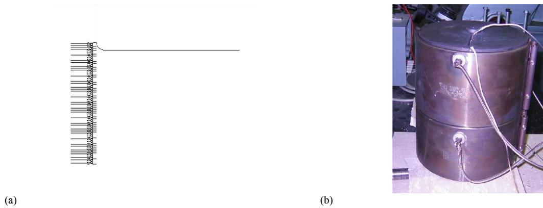
Figure 1: a) Schematic view of the die and sheet mesh and b) forming dies for bulging test
