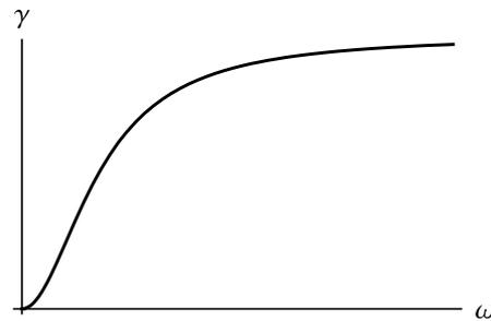
Figure 5. Dependence of the acoustical absorption factor on frequency
