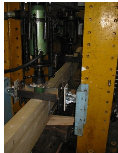
Figure 7. Stabilization against overturning (lateral buckling)
