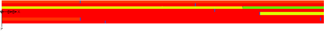
Figure 15. Distribution of averages of Young's moduli within the beam with small deflection of 16.87 mm
