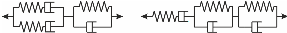
Figure 4: Burgers body and Kelvin-Voigt body in series (left). This model is mechanically equivalent to a serial connection of Hooke element, Newton element and two Kelvin-Voigt bodies (right).
