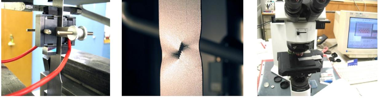
Figure 6. A specimen in the testing machine (*left*), deformation of the zone with artificial defects (*center*), measurement instrumentation (*right*)
