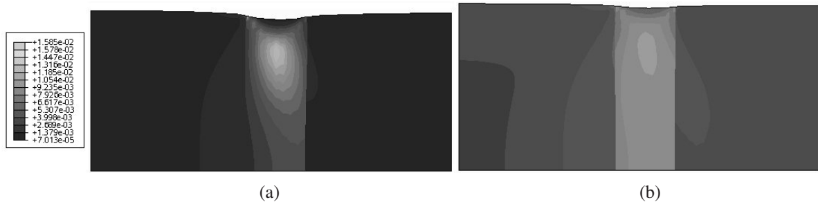
Figure 12: Distribution of void volume fraction at 7595.4 hrs calculated in the case of (a) original d as shown in Table 1 and (b) twice of original d
