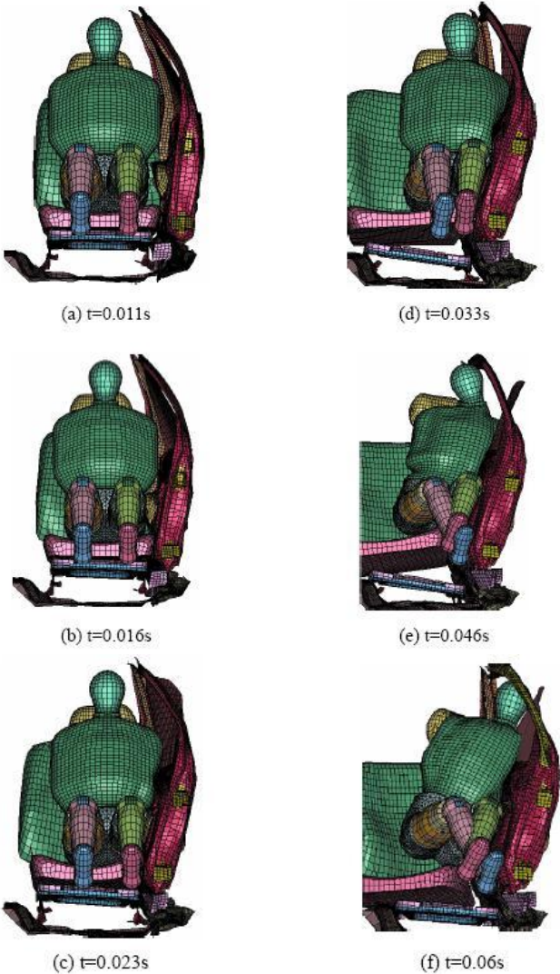
Figure 7. A simulated impact sequence of side impact test
