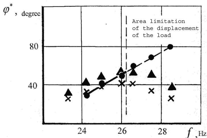
Figure 3. Dependence of the greatest possible deviation by the angle  $\varphi^*$ , providing the return of the pendulum to the stable upper vertical position of the quasi-equilibrium on the oscillation frequency of the axis of its suspension.
