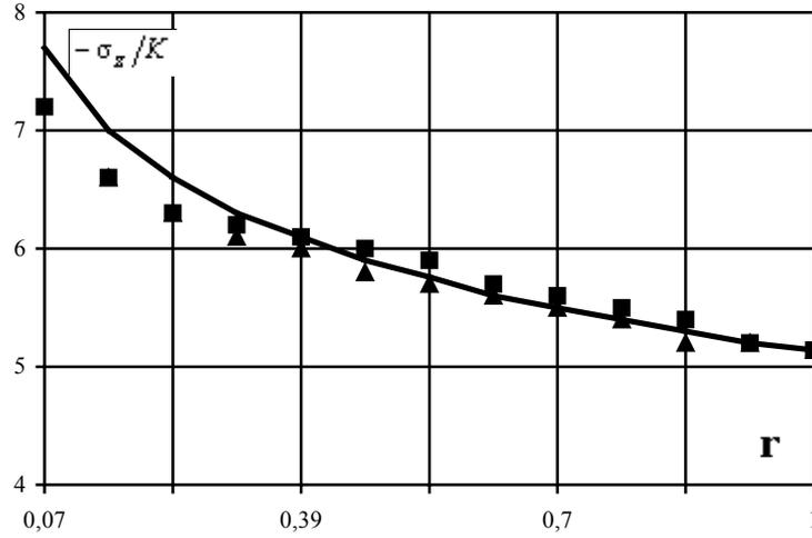
Figure 3. The distribution of  $(-\sigma_z / K)$  for a flat rigid cylindrical punch: The line (—) is calculated by (16); The sign (▲) is for numerical results of A.J. Ishlinsky (Ishlinsky, 1944; Ishlinsky and Ivlev, 2001); The sign (■) is for numerical results of R.T. Shield (Shield, 1955);
