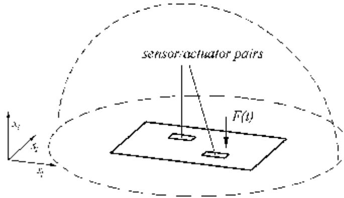
Figure 2. Smart plate structure coupled with acoustic half space
