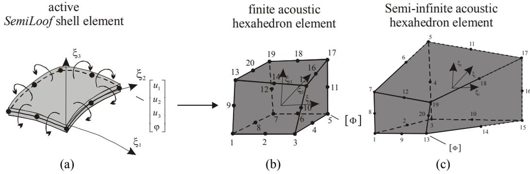
Figure 1. Coupling of shell elements and acoustic hexahedron elements: (a) piezoelectric *SemiLoof*-type shell element, (b) acoustic hexahedron element, (c) semi-infinite acoustic element
