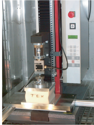
Figure 1: Buckling of a cubic test specimen at a uniaxial compression test
