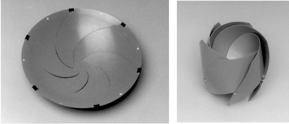
Figure 2: Small scale model, deployed and packaged.
