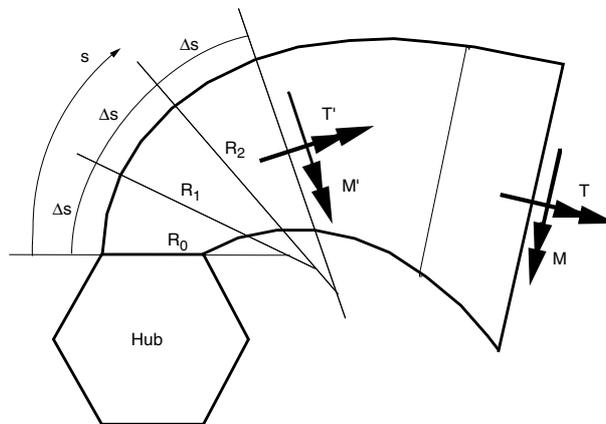
Figure 6: Cutting pattern for cones of increasing height.
