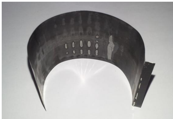
Figure 5. Damage of the sliding surface in the top foil
