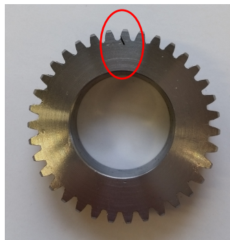
Figure 2: Artificially cracked planet tooth
